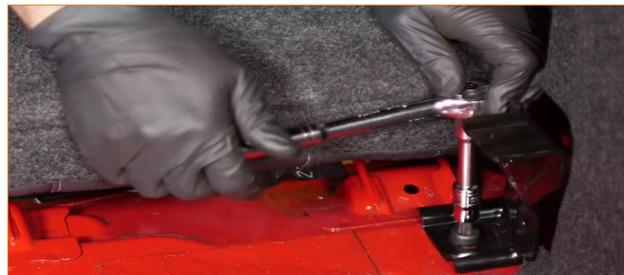
04. Lower the Mishimoto strut brace into place over the seat mounts. Secure the strut brace and the seat mounts using the hardware you just removed. (2x T50 Torx bolts)
