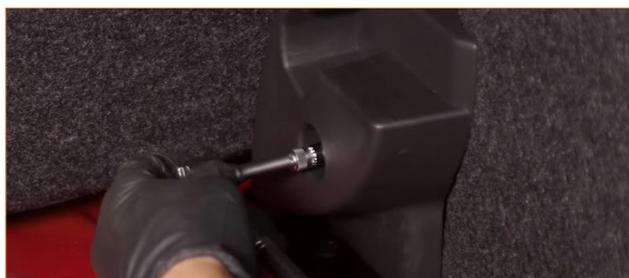
03. Remove the two bolts that secure the outer seat mounts. (2x T50 Torx bolts)
