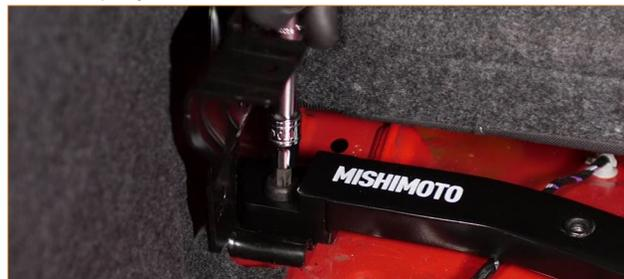
05. Reinstall the false-floor mounts, and secure them with the original hardware. (2x 8mm bolts)
