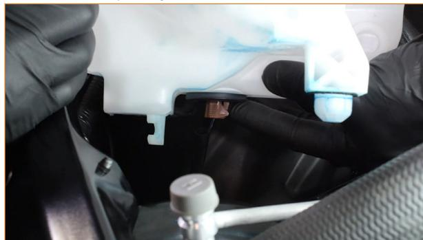
04. Disconnect the gray electrical connector from the side of the tank. Then release the washer fluid line from the tank.
