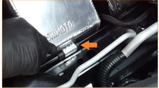
**11.** Install the washer pump to the Mishimoto tank. Simply push it in until it is fully seated, and reconnect the electrical harness.
