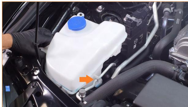
03. Lift the washer tank up a few inches to access the electrical harness on the bottom of the tank. Separate the brown connector from the fluid level sensor by depressing the tab and pulling the connector out of the sensor.
