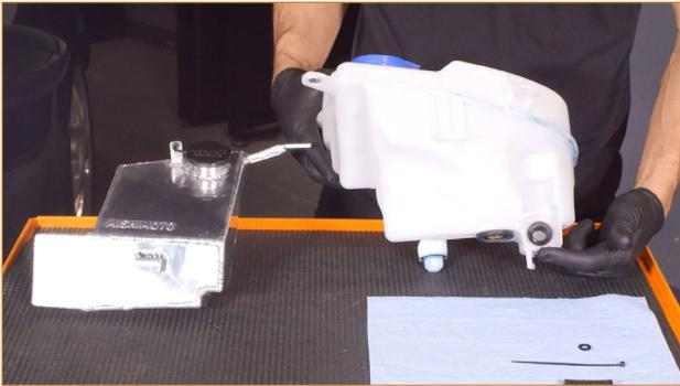
**08.** Install the washer grommet in the Mishimoto tank.
