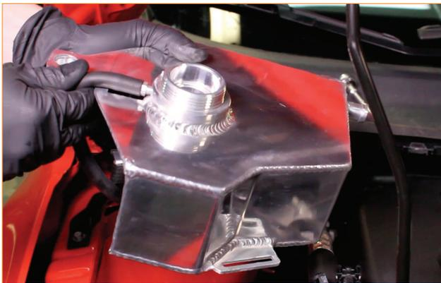
17. The slotted brackets on the Mishimoto tank will slip over the stock mounting pegs. The hole on the top of the tank installs over the stud on the strut tower (where the AC line bracket is mounted).
