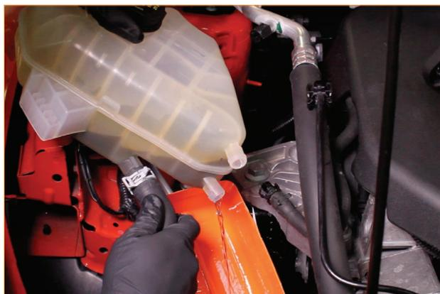
8. Remove the upper coolant line by squeezing the clip and pulling the line out of the bottle.
