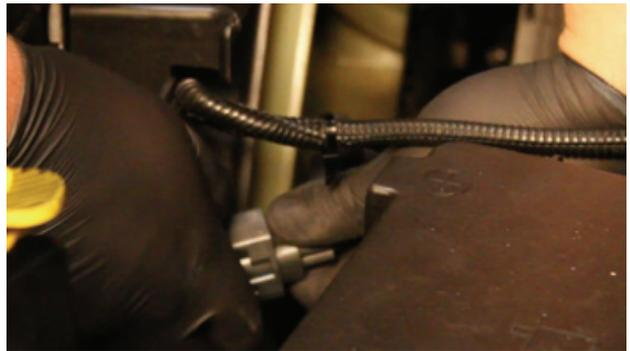
9. Undo push clip that holds the fan shroud connection to the plastic fan shroud.
