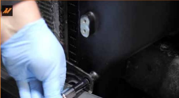
18. Reconnect the cold-side intercooler pipe and boot to the intercooler. Tighten the clamp once the boot is seated properly on the intercooler.
