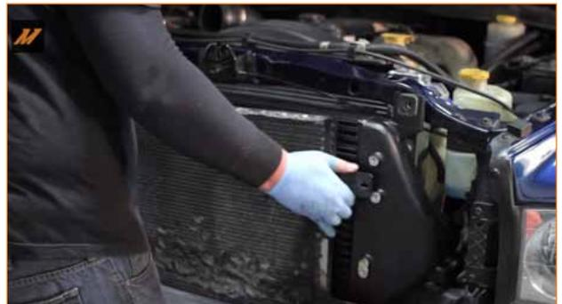
15. Move the AC condenser back to its proper position in front of the intercooler.
