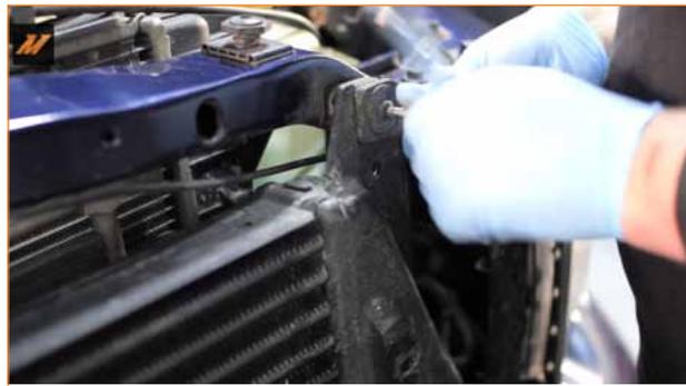
8. Remove the two T30 Torx bolts that secure the intercooler to the upper radiator support.
