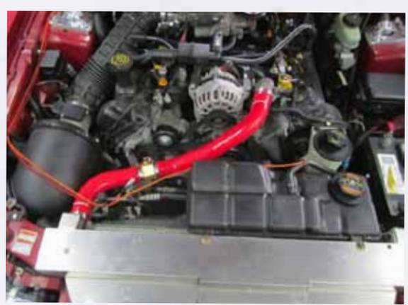
Figure 2: PLX sensors were attached to the vehicle to obtain inlet and outlet temperatures from the radiator
