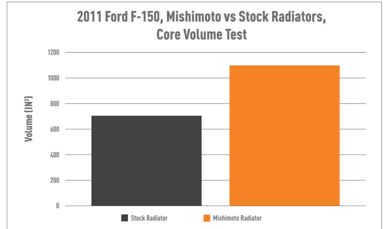
FIGURE 4: The Mishimoto radiator features an increase in core volume.
