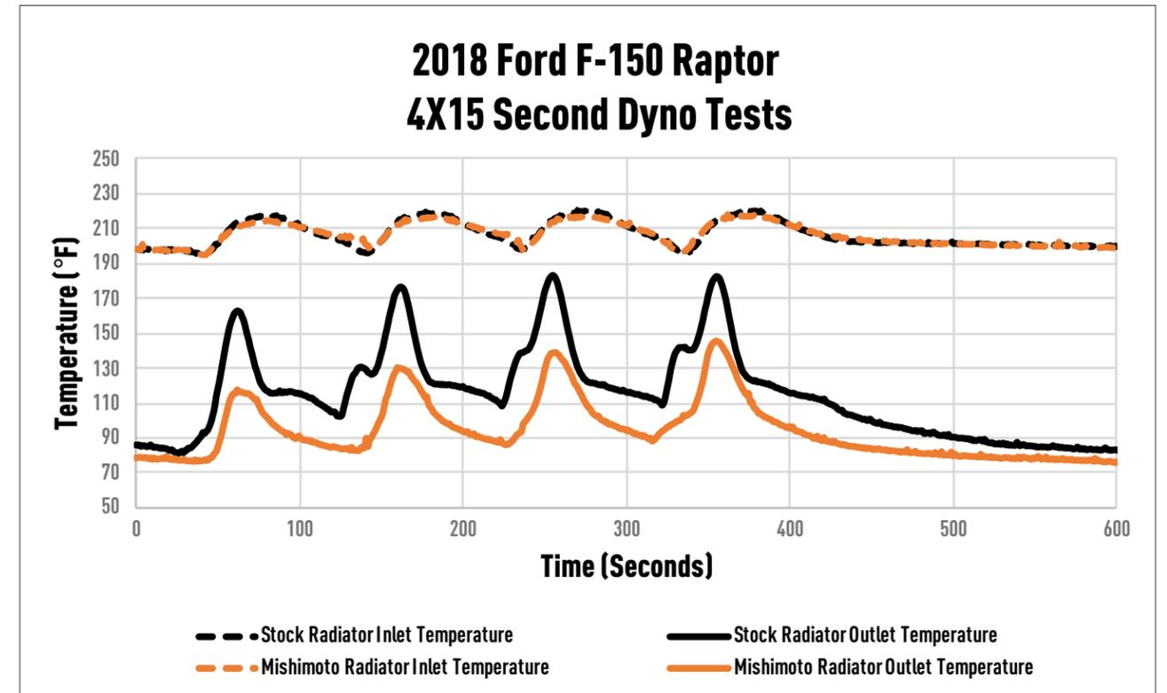
FIGURE 5: This is the Mishimoto Radiator vs the Stock Radiator. Notice how the Stock outlet rises faster during the dyno pull while the Mishimoto outlet is slower.
