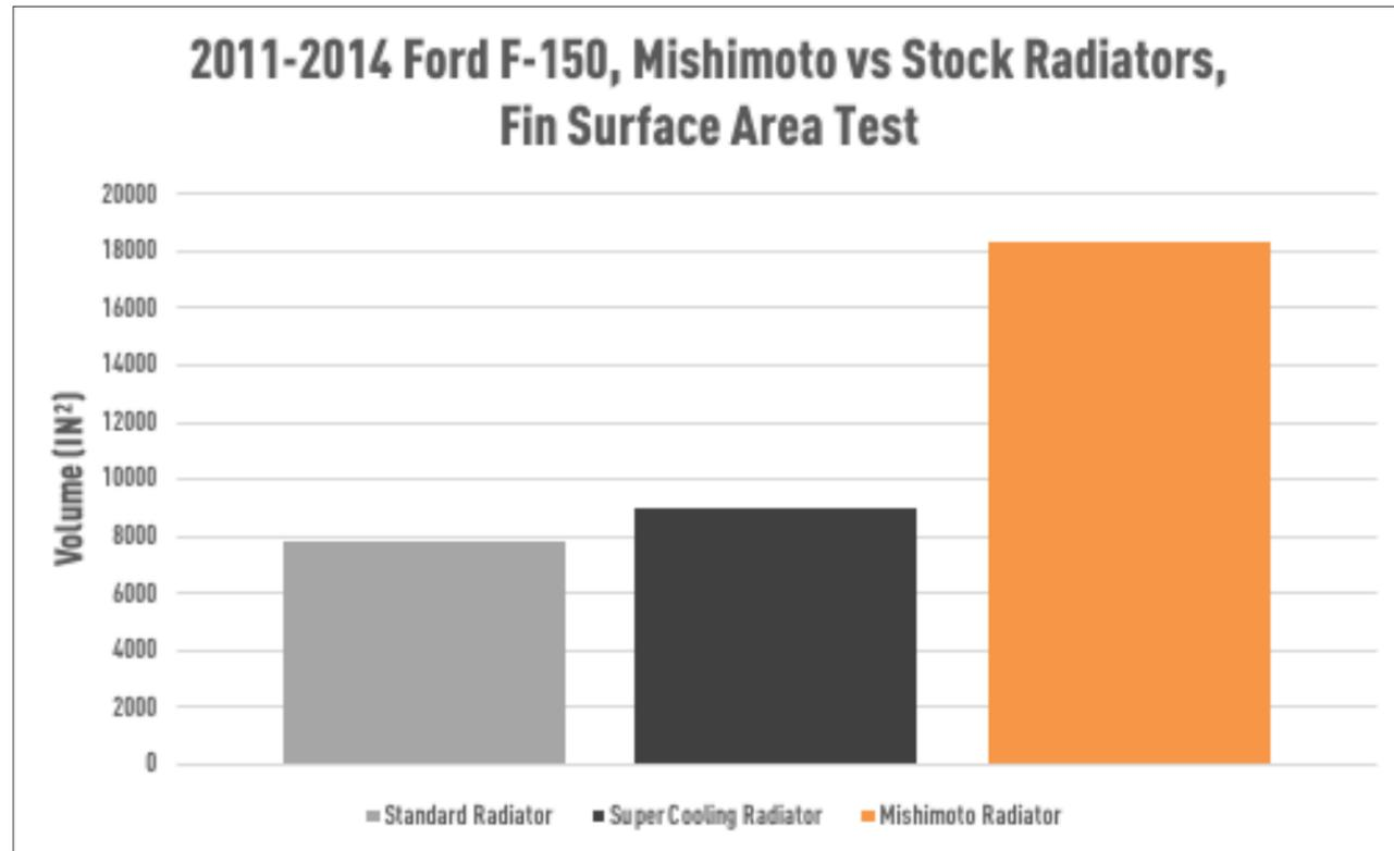
FIGURE 3: The Mishimoto radiator features an increase in Fin Surface Area, which promotes greater heat transfer.
