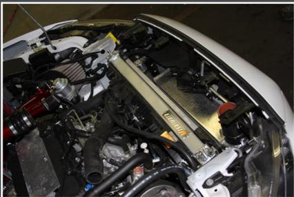
6. Reinstall the core support, watching the middle brace and bumper tabs. (It's easier to run and clip in the harnesses while the radiator support is loose).
