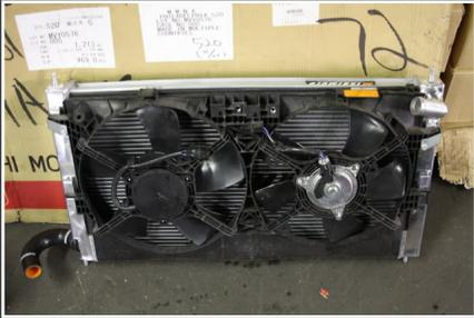
3. Slide the radiator into engine bay on the driver's side first to get the u-shaped hose to clear the side.
