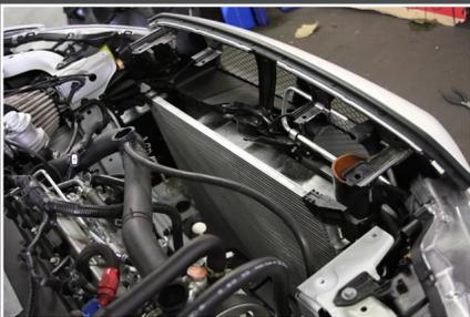
16. Stock Fan assembly has 4 clips and (2) 10mm hold downs.
