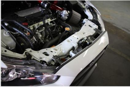
4. Remove (4) 10mm bolts from bumper tabs, (3) 10mm hood latch bolts and pop the cable out (Unplug harness directly behind core support - 2 wires).
