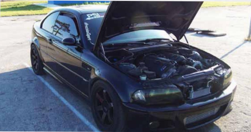
**Figure 1:** Test vehicle: Notice the additional heat exchangers in front of radiator.
