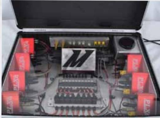
**Figure 4:** PLX sensor modules were used to monitor engine pyrometers.
