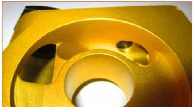
6. Notice that no Teflon® tape is inside the npt port area.
