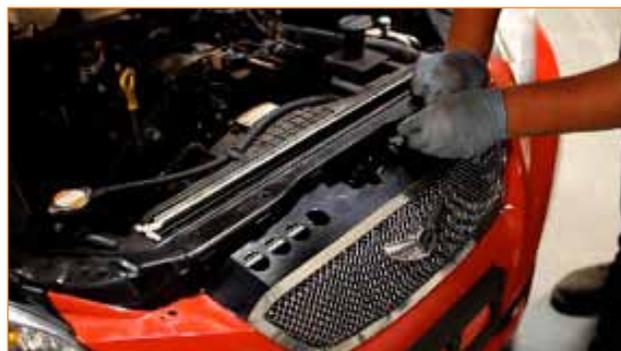
8. Reinstall the front air dam using four pop clips.
