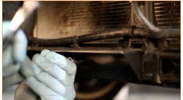
5. Bolt the oil cooler to the mounting bracket using the supplied four 10mm bolts.
