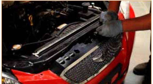
8. Remove the front bumper by pulling on the corners of the bumper to undo the retaining clips.
