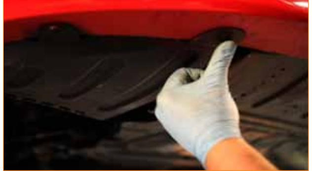
6. Remove the front splash pan by removing the four 10mm bolts.
