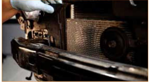
4. Bolt the oil cooler bracket to the support beam using the two supplied 10mm bolts.
