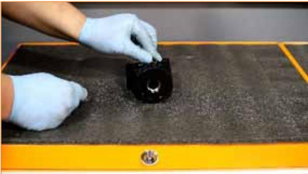
2. Apply oil to the O-rings on the oil filter housing.
