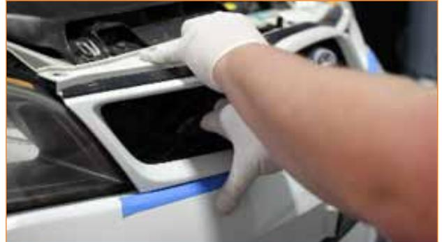
6. Remove the two hidden pop clips from the bumper. The clips are behind the side grille inserts.
