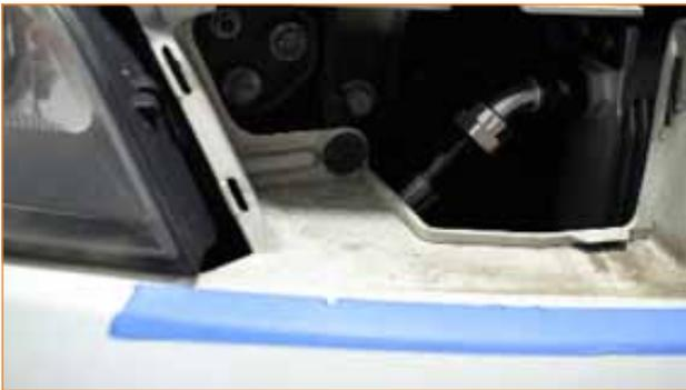
4. Reinstall the two hidden pop clips on the bottom of the front bumper, then reinstall the side splash shields and secure them to the bumper using six pop clips.
