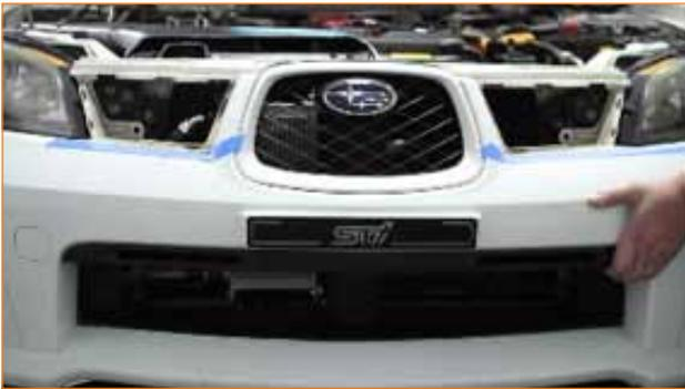
2. Reinstall the six pop clips that hold the top of the bumper to the upper radiator support.
