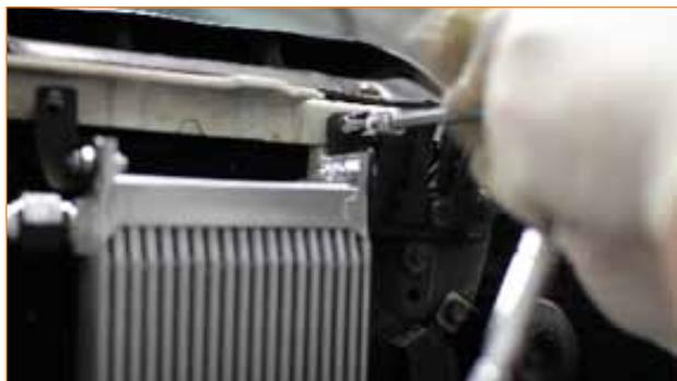
10. Using the supplied Mishimoto hardware, secure the upper left bracket of the oil cooler to the upper radiator support.
