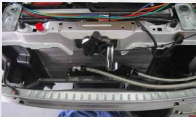
Figure 5: The lower placement of the oil cooler showed a 35°F temperature drop over stock at cruising speeds.
