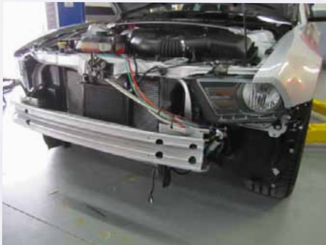
Figure 4: The first mounting location showed a 20°F temperature drop over stock. This was considered adequate but not quite good enough.
