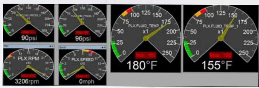
Intake air temperatures were taken from both the inlet and outlet of the intercoolers using PLX K-type thermocouples. Boost pressure was also tested to ensure that no dramatic pressure drop occurs due to the larger Mishimoto intercooler.
