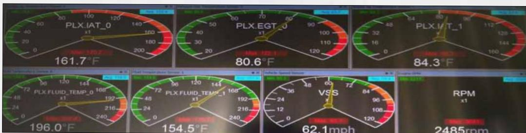
Intake air temperatures were taken from both the inlet and outlet of intercoolers using PLX K-type thermocouples. Boost pressure was also tested to ensure that no dramatic pressure drop occurs due to the larger Mishimoto intercooler.
