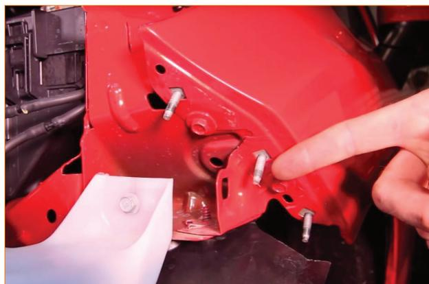
10. Remove the bumper cover by sliding it forward, away from the vehicle.
