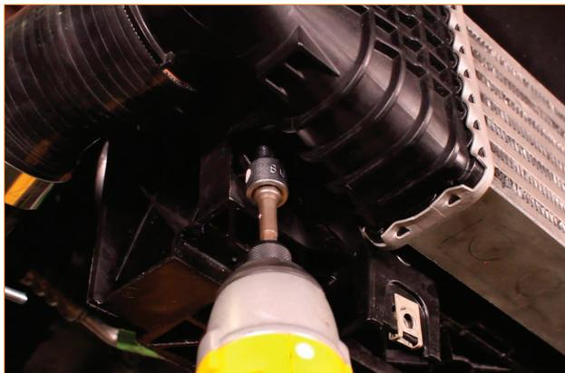
14. Remove the intercooler from the vehicle. The top of the intercooler is held in by two grommets. Pull the intercooler down, and slide it out of the couplers.
