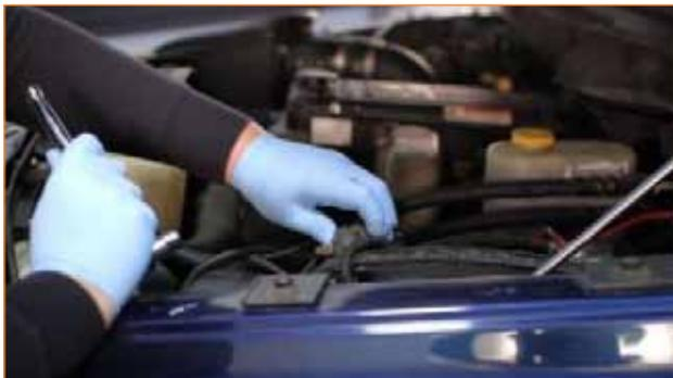
11. Remove the upper radiator support beam. Slide the beam to one side and lift the opposite end upward to detach it from the lower radiator support. The hood latch cable will still be attached to this component, so place the beam carefully on top of the engine and out of the way.
