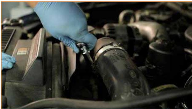
2. Remove the coolant overflow hose from the reservoir and place it to the side to allow for clearance when removing the pipe.
