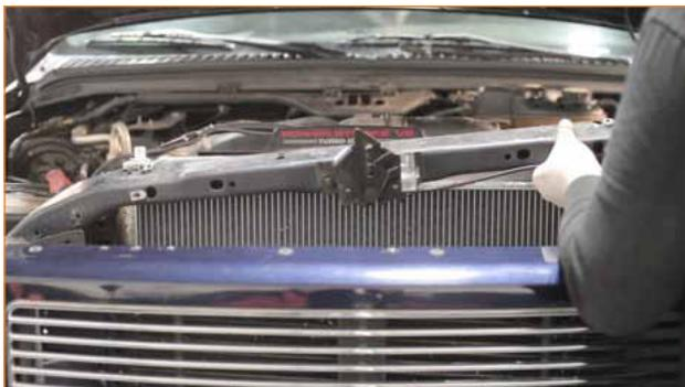
4. Loosely install the eight 13mm bolts for the upper radiator support beam until the beam is lined up in the factory location. Make sure the bolt heads line up with the paint marks from the factory installation. Once everything is lined up, fully tighten the upper radiator support bolts.
