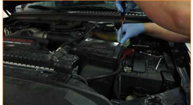
3. Remove the nine pop clips that hold the upper fan shroud to the grill and radiator support. Once the pop clips have been removed, the upper shroud can be detached.
