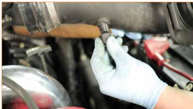
13. Start the vehicle and check for any leaks in the charge-air system.
