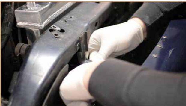
7. Reinstall the three pop clips securing the wire harness to the top of the radiator support.
