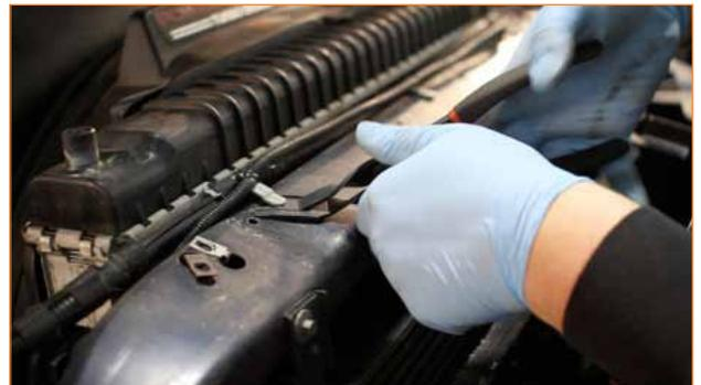
7. Remove the two 8mm bolts that secure the AC condenser brackets to the upper radiator support.
