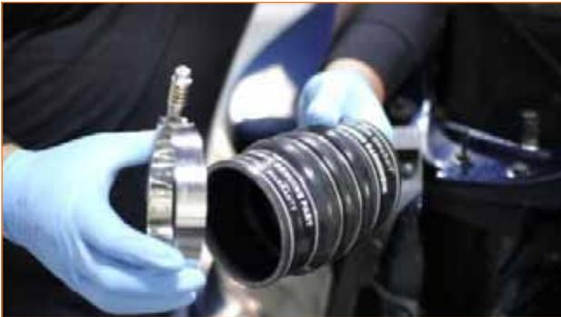
5. Insert the Mishimoto hot-side intercooler pipe into the boot on the intercooler. Once in position, slide a 4" constant-tension T-bolt clamp over the pipe and onto the boot. Tighten the clamp to secure this pipe.
