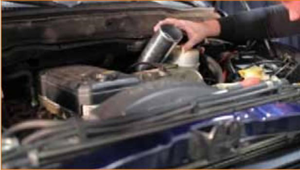
2. Install the silicone boot that connects the Mishimoto cold-side intercooler pipe to the intake manifold. This boot features a transition from 3" to 3.5" with the smaller side attaching to the intake manifold. Use one 4" clamp and one 3.25" clamp to secure this silicone boot.
