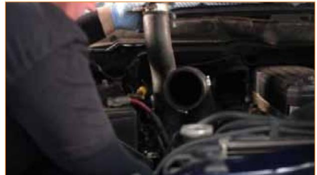
6. Using a 10mm socket or wrench, remove the 10mm bolt and the clamp that secures the cold-side intercooler pipe to the intercooler.
