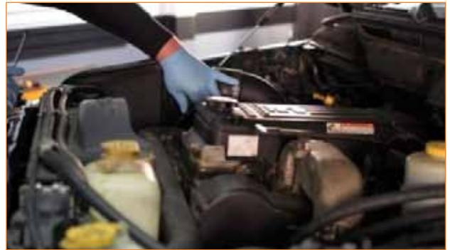
3. Loosen the clamp connecting the airbox to the turbocharger, and remove the airbox assembly from the vehicle.
