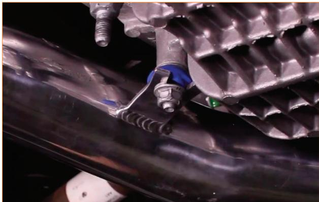
9. Now go back and tighten all the clamps on the hot-side pipe. (3x 10mm clamps)
