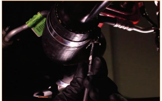
4. Loosen the clamp that secures the hot-side pipe to the turbocharger outlet, and remove the pipe from the vehicle.
