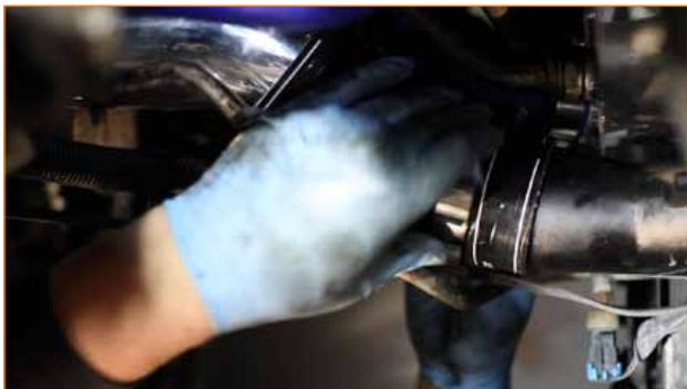
2. Connect the cold-side pipe and boot to the intake.
