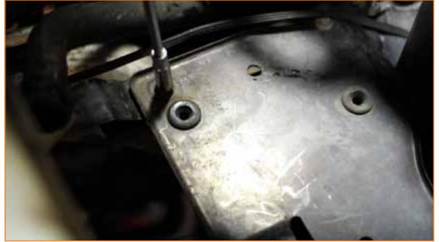
6. Unbolt the airbox-mounting bracket from the coolant reservoir by removing the single 10mm bolt.
