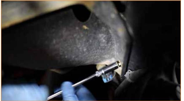
8. Disconnect the cold-side boot and pipe from the intercooler.
