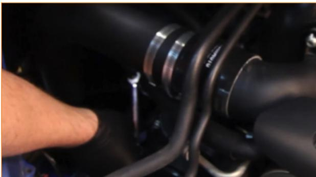
3. If the vehicle is equipped with the stock air intake, simply remove the post MAF hose and set aside. (2x worm-gear clamps)
