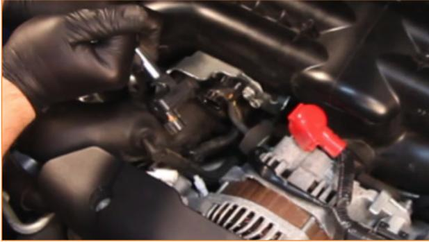
13. Remove the plastic sensor housing located to the right of the boost solenoid. (1x 12mm bolt)
