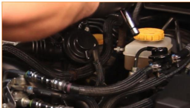
8. Loosen the hose that connects the intercooler to the throttle body. (1x worm-gear clamp)
