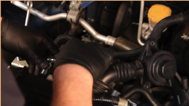
20. Disconnect the throttle-body electrical connector behind the engine.
