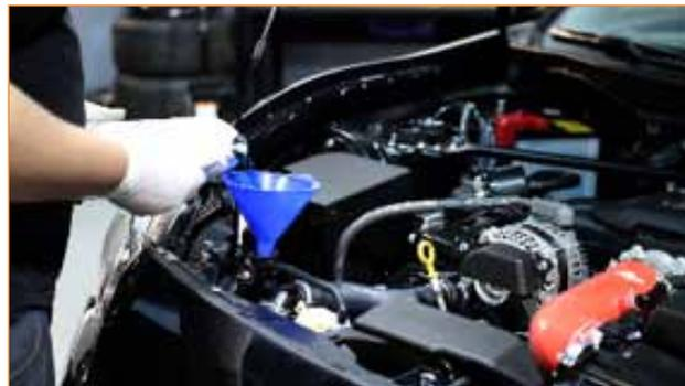
15. Start the vehicle and set the heat to high to purge any air from the cooling system. Allow the vehicle to reach operating temperature and check for any leaks in the system.
