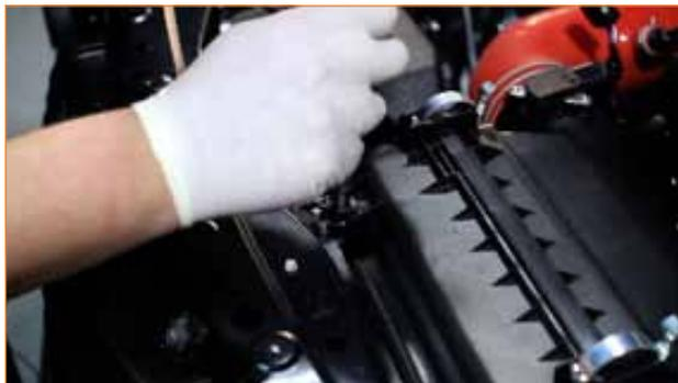
9. Remove the intake box assembly.
