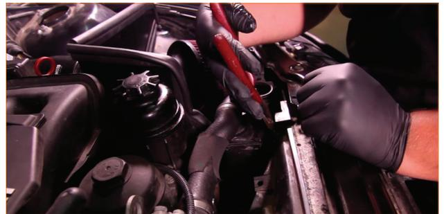
06. Disconnect both electrical connectors from the fan shroud.
