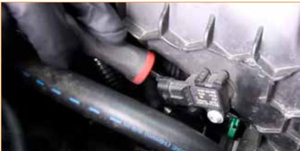
**09.** Loosen the worm-gear clamp that secures the charge pipe to the throttle body. (7mm socket or flathead screwdriver)
