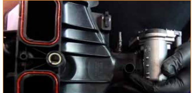
**CAPTION:** The PCV port on the back of the intake manifold is not visible while the intake is installed on the vehicle.
