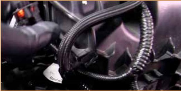
**07.** Free the vacuum line from the three clips that secure it to the manifold.
