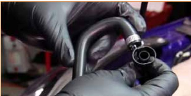
20. Lead the other end of this hose (the end without a fitting) toward the driver side. It should pass over the starter motor and behind the engine harness, exiting in front of the transmission.
