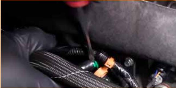
18. Remove the black plastic fitting from the PCV hose by pulling it out.
