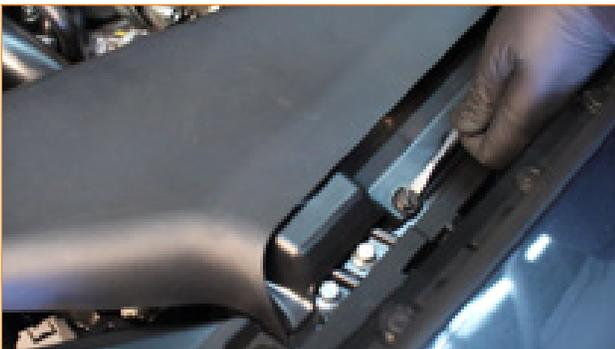
2. Loosen the intake hold-down bracket on the passenger side fender at the top of the airbox (2x 10mm nuts)
