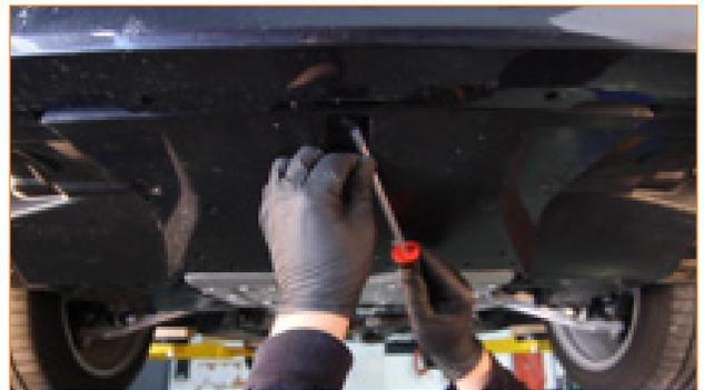
6. Remove the clips holding the undertray to the aluminum plate (4x small pop clips)
