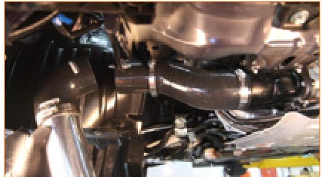
2. Tighten the engine side clamp (1x worm-gear clamp)
