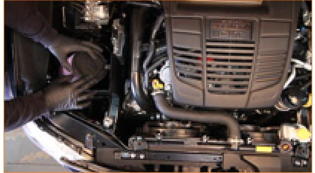
6. Tighten down the clamp (1x worm-gear clamp)
