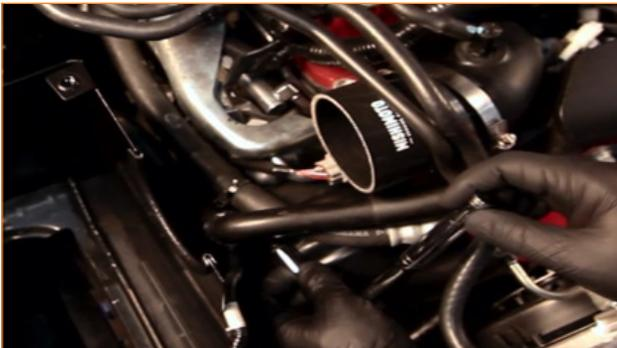
7. Install the Mishimoto-supplied bracket. (1x 10mm bolt)
