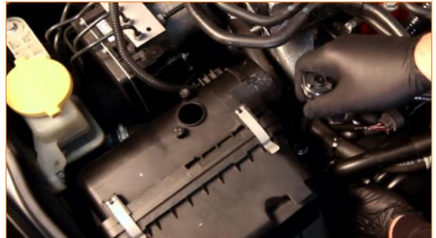
9. Unscrew and remove the rear portion of the headlight.
