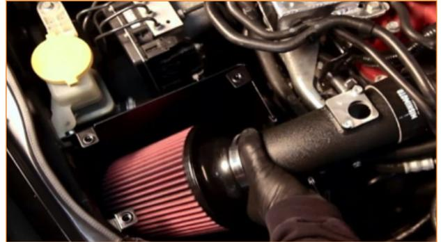
11. You may now tighten and adjust the two worm-gear clamps.
