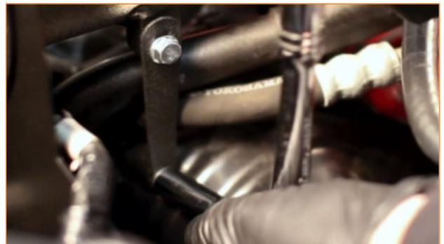
13. Reuse the bolt for the timing cover to secure the pipe and bracket.
