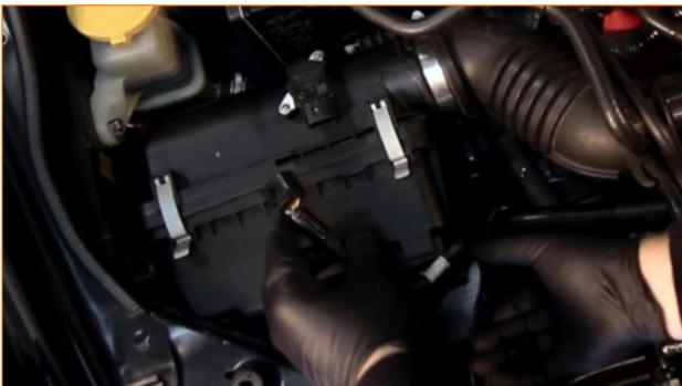
3. Using a Phillips screwdriver, remove the two screws securing the MAF sensor, and then remove it from the vehicle.
