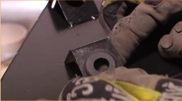
12. Install the mounting bracket onto the Mishimoto airbox using the supplied Allen bolts. (2x 4mm Allen bolts)
