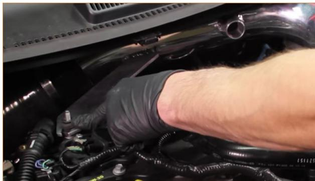
17. Install the nut that secures the intake, but do not fully tighten it yet. (1x 10mm nut)
