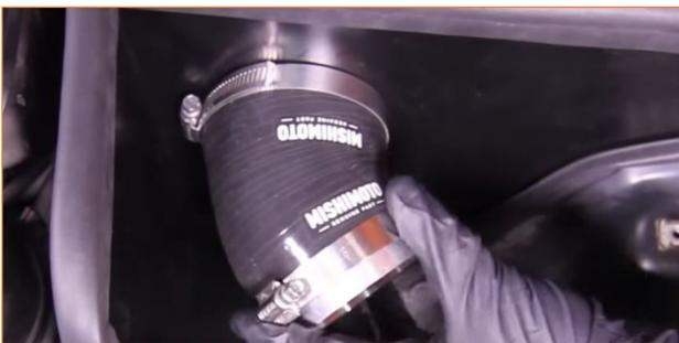
10. Install the air filter over the aluminum adapter. Secure the air filter with the worm-gear clamp. (1x worm-gear clamp)
