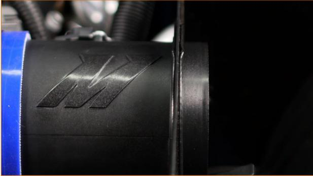
22. Connect the electrical harness to the MAF sensor, and secure it with the red lock tab. Adjust the MAF housing to ensure that the harness is not under tension. Secure the induction hose to the MAF housing with the worm-gear clamp that you installed earlier.
