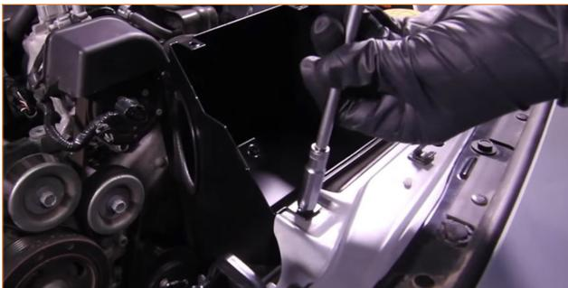
**09.** Lower the Mishimoto air filter into the airbox. Insert the MAF housing through the large hole on the airbox and into the air filter. When properly installed, the connector on the MAF should face toward the engine.
