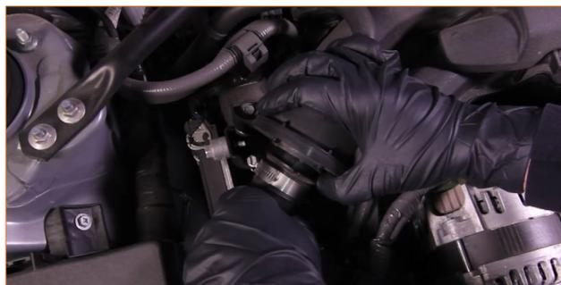
05. Remove the three bolts that secure the stock airbox to the vehicle, and then remove the airbox assembly. (3x 10mm bolts)
