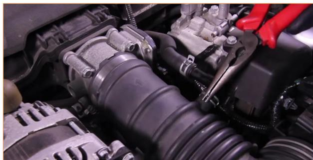
03. Loosen the two clamps that secure the induction hose to the throttle body and airbox. (2x worm-gear clamps)
